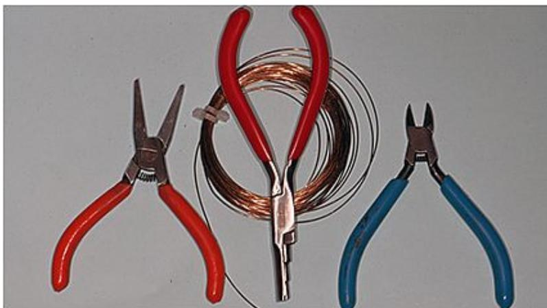
Right to left: Flat Nose Pliers, Jewelry Looping Pliers, Wire Cutter with copper tinted SS wire in the background.
