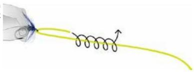
2. Bring the tag end of the line back through the first loop formed behind the eye. If you pull the tag end tight (close the knot) at this point, you have tied the Clinch Knot. However, if you do not close the knot, but instead pass the tag through the big loop as illustrated below, wet the knot, then pull the tag end tight and close the knot, you just tied the Improved Clinch Knot. Seat the knot by pulling on the standing line, and by pulling the tag end.
