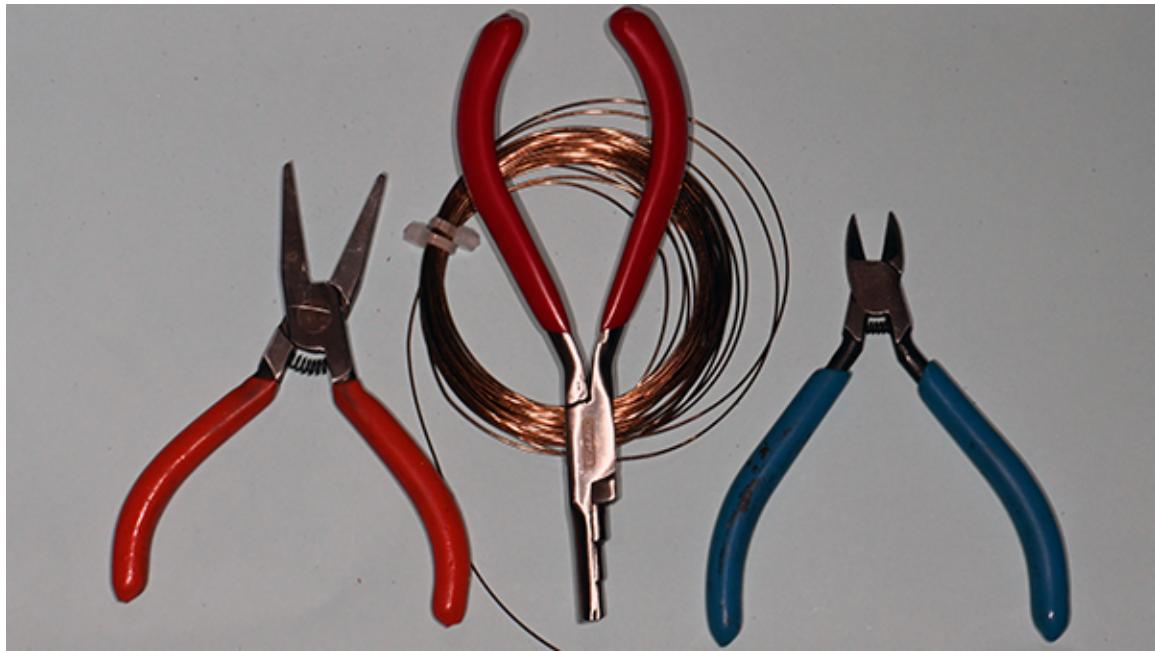
Right tool- Flat Nose pliers: Center tool is Looping pliers: Far left is a pair of Wire Cutters
